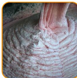
1. Crosslinking process which gels and increases water resistance.
