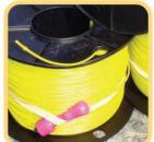
Colour coded connector will accept up to eight (8) shock tubes.
